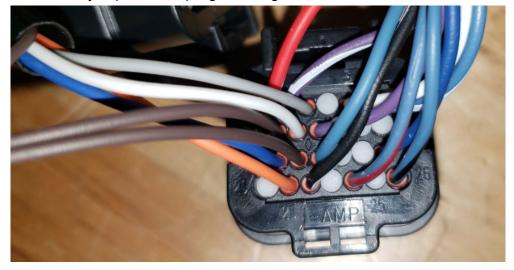
Once all 6 wires are inserted fully, push on the 2 small white tabs to lock the connector so the wires can't be removed or inserted. Very little force needs to be applied to lock the connector. If the white tabs don't easily slide back into place, one or more of the
