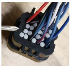
• Remove these 6 cavity plugs. They are only held in by the friction of the seal.
