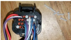
• Find the large white lock on the side of the connector. Push on this lock and you will hear a click. When this is unlocked, it allows wires to be removed and inserted. Be careful not to pull on any existing wires, as they can be pulled out with little force.
